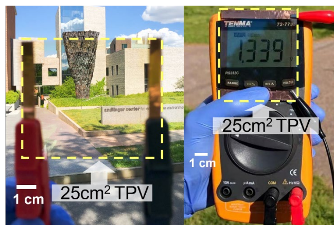
Figure 2. Photographs taken outdoors of a 25 cm 2 TPV and its photovoltage shown on a multimeter under ambient sunlight.
